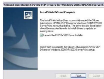
When the installation finishes, be sure to click the box labelled 'Launch the CP210x VCP Driver Installer' and click finish.
