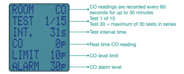
Otherwise Room CO tests automatically end after the pre-set time.
