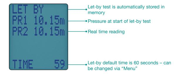
If let-by test fails rotate dial to another position to stop the test.
